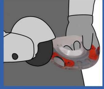
Adjust the horseshoe to the hoof with an angle grinder or belt grinder.
