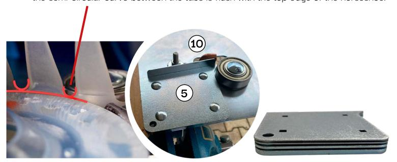
IV. Put the nozzle (no. 4) on your hot-air gun (see no. 4). Position the hot-air gun in its mount under the welding board (no. 10). Use the open-end spanner wrench 10mm (no. 3) to fasten the hot-air gun. Tighten the screw hand-tight.
